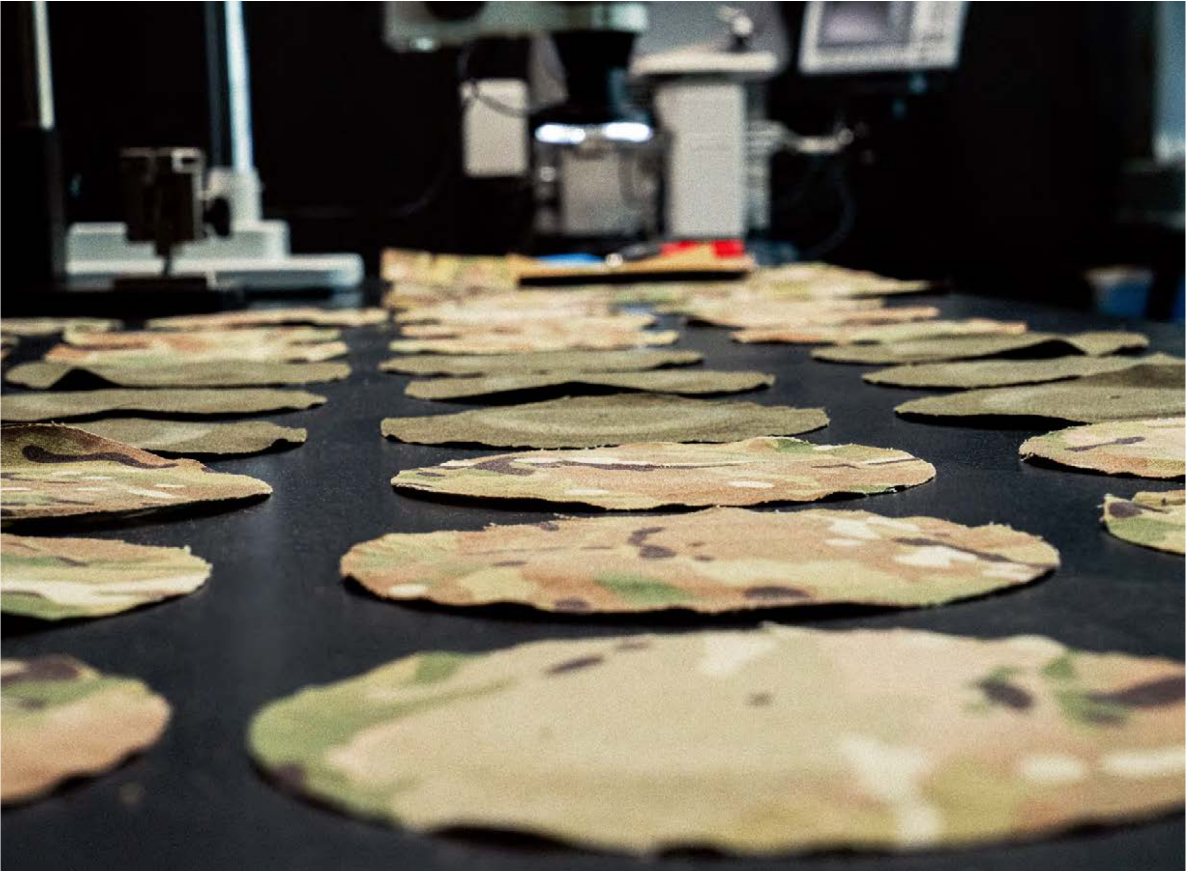
MultiCam® fabric abrasion testing
