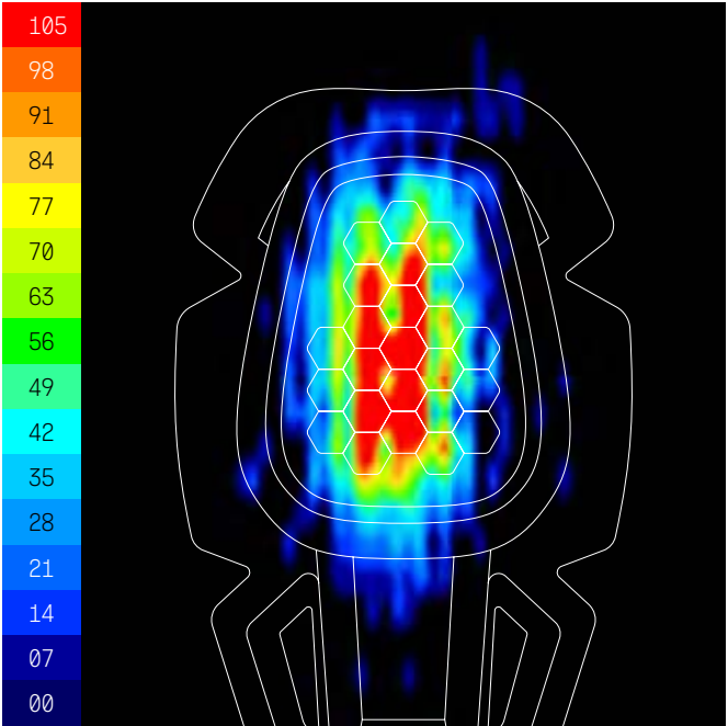
AIRFLEX™ IMPACT COMBAT KNEE PAD pressure sensor map in PSI
